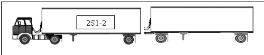
(LSIORB Class – Large Truck) FHWA Class 11 — 5 or Less Axles, Multi-Trailers
